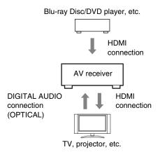
2. Connect the audio output from the TV to the **OPTICAL IN 2** jack of the AV receiver using an optical digital cable.
