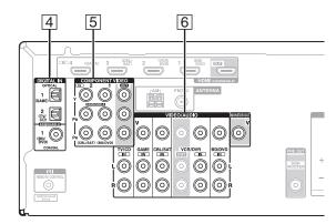
Connect your components to the appropriate jacks. The default input assignments are shown below.
